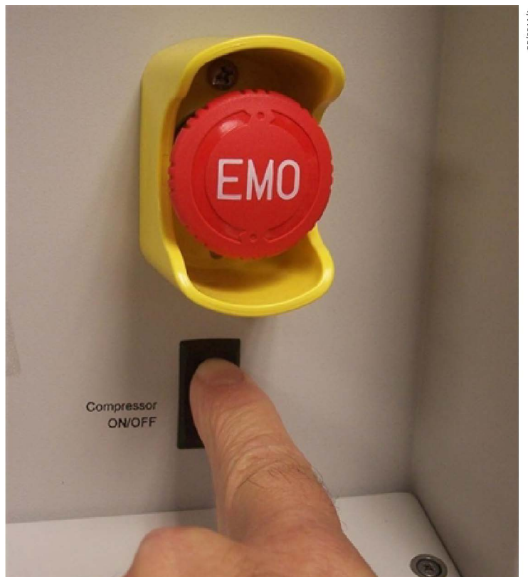
Figure 91 Set compressor switch to ON (optional EMO shown)
