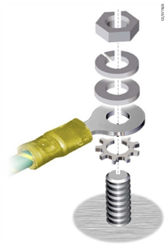
Figure 49 Ground washer stack sequence
