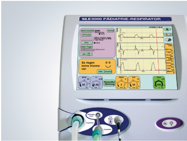
Figure 2: Neonatal Ventilator with High Frequency Oscillation: SLE5000
