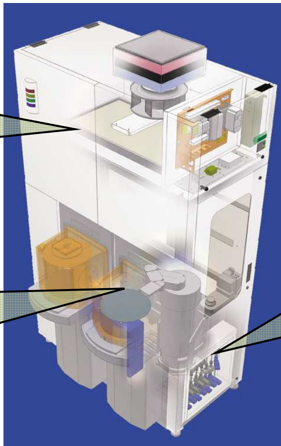
Typical 300mm Equipment Front End Module (EFEM) Solution
